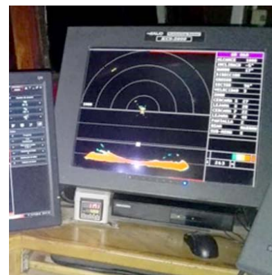
The WESMAR sonar is normally set at 1000 meter range when fishing hake.
