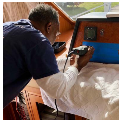
Ray McClue from YEP prepares the instrument panel for the DSP5000 control station..
