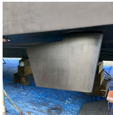
The new OLOH stabilizer fins each measured 7.5 sq. ft. to gain optimal performance.
