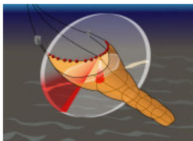
Two views: 360 degree net profile and down sounder for monitoring fish, footrope, and changes to the net.
