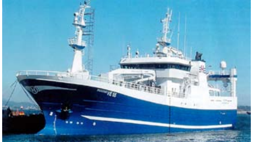
Huginn pictured at the Asmar Shipyard in Chile. She is a 68-meter long seiner/trawler that will be fishing herring, capelin and blue whiting in the North Atlantic Ocean for her Icelandic owner Gudmundur Huginn.
