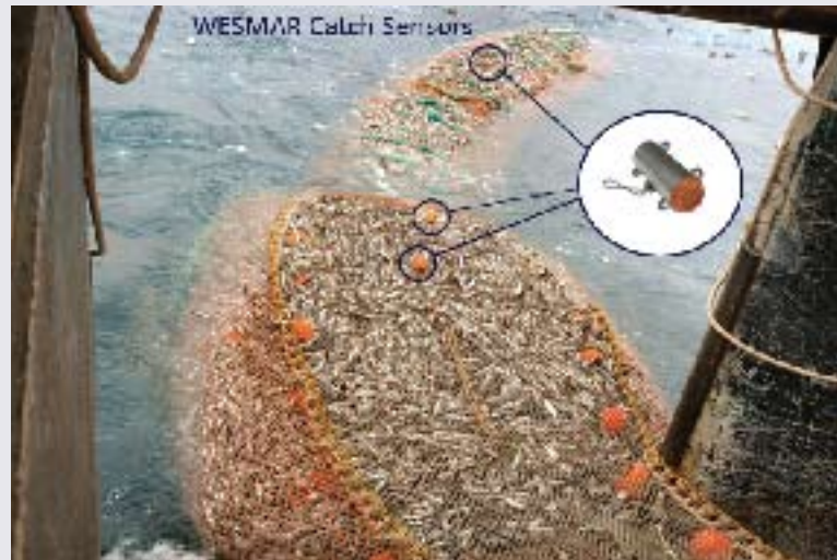
A full bag of Alaska Pollock ready to board the C/P Arctic Storm. Captain Styke found this 100 + ton catch with the WESMAR HD850 sonar and used the WESMAR TCS780 Trawl Sonar to profile the opening of the net. WESMAR Catch Sensors monitored the filling of the cod end.
