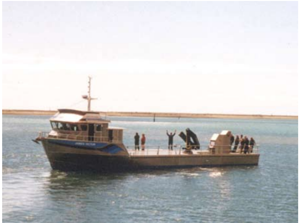
The Vessel James Victor, a 30-meter barge in Nelson, New Zealand, uses a WESMAR counter rotating 37kw side thruster to give the vessel the maneuverability required to move around the spat lines and hold close to the line catcher.
