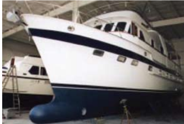
American Boat Works' bow thruster installation and bulbous bow addition on 52' DeFever.
