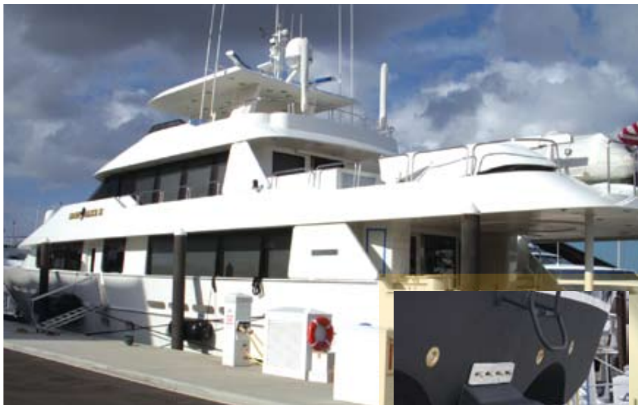
The 130' M/Y Mary Alice II is a stately luxury yacht with 5 staterooms that accommodate 10 guests comfortably. The Mary Alice was sold with a WESMAR Bow Thruster and the new owners decided to add a WESMAR Stern Thruster as well.
