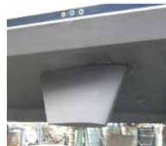
It was smooth riding for the 76-foot Rayburn after being fitted with WESMAR 9-sq foot fins.
