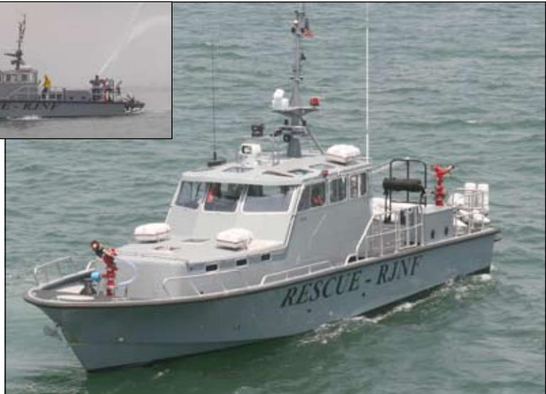
*The all stainless steel, WESMAR V2-12 hydraulically driven dual prop counter rotating bow thruster system on board a 17 meter (60 foot ) Search and Rescue (SAR) vessel built for the U.S. Navy Office of Foreign Military by Willard Marine has been in service since 2008 and provides an enormous amount of capability to maneuver in close quarters and hold steady to position during critical Search and Rescue missions.*
